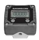
Oval gear in-line meter for use with lubricants and diesel. Meter includes an electronic register powered by two "AAA" Alkaline batteries. Meter display is multi-function, showing the volume dispensed per delivery and has a permanent and a resettable (trip function) totalizers. The display can be programmed to show delivery in liters, quarts, pints, and gallons. The assembly is protected by a TPE shroud.
